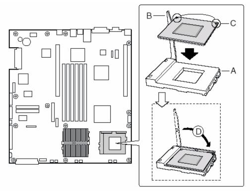
Figure 21: Installing the Processor Terminator
